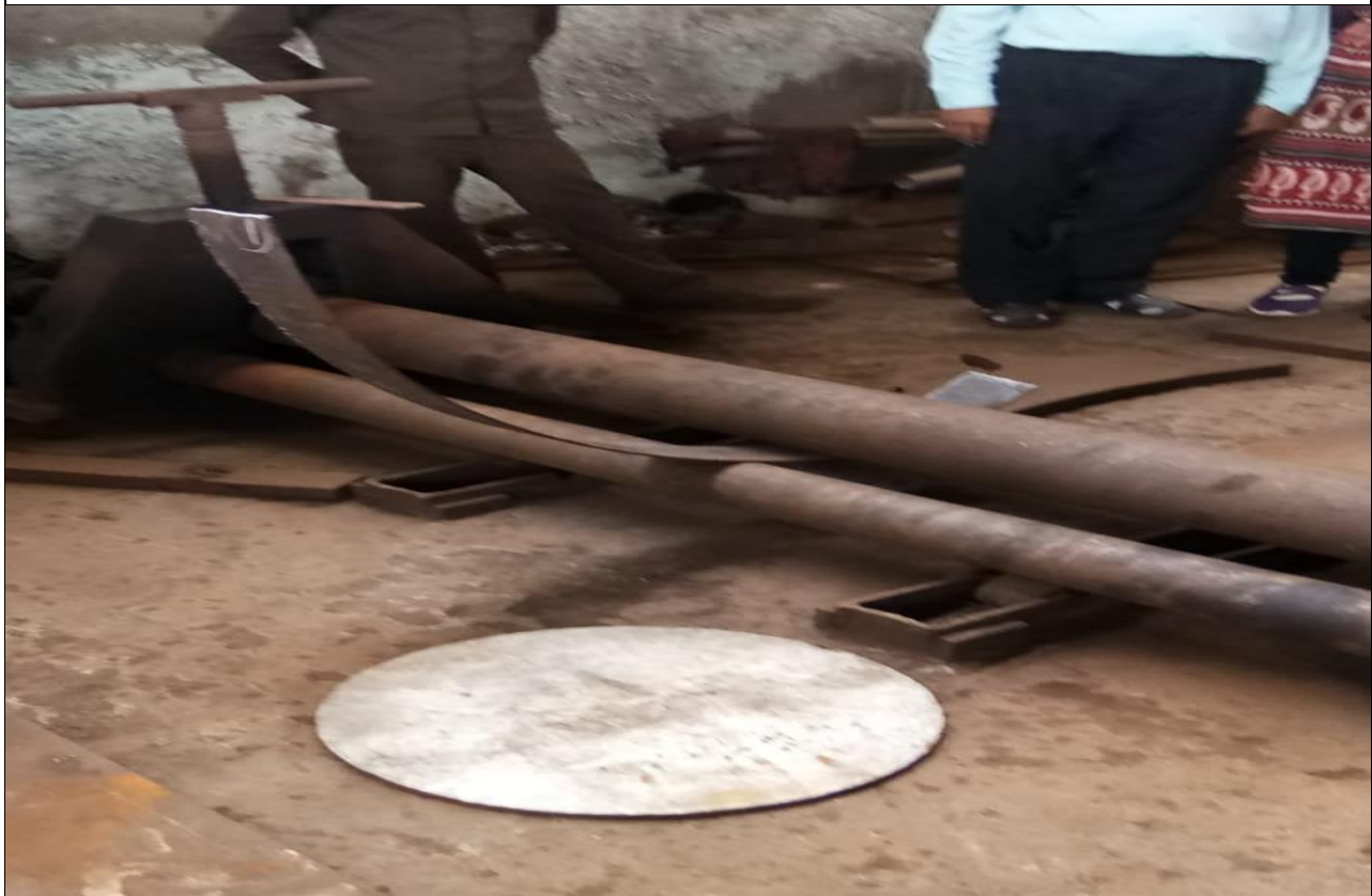
Mr. B A Patil explaining how a plate is given a circular shape to form head
